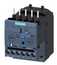
Overload relay 4...16 A Electronic For motor protection Size S00, Class 5...30 Contactor mounting Main circuit: Screw Auxiliary circuit: Screw Manual-Automatic-Reset Internal ground fault detection
