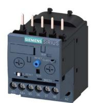
Overload relay 1...4 A Electronic For motor protection Size S00, Class 5...30 Contactor mounting Main circuit: Screw Auxiliary circuit: Screw Manual-Automatic-Reset Internal ground fault detection
