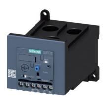
Overload relay 32...115 A Electronic For motor protection Size S3, Class 20E Stand-alone installation Main circuit: Straight-through transformer Auxiliary circuit: Screw Manual-Automatic-Reset
