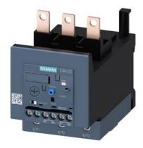
Overload relay 32...115 A Electronic For motor protection Size S3, Class 20E Contactor mounting Main circuit: Screw Auxiliary circuit: Screw Manual-Automatic-Reset
