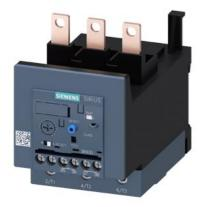
Overload relay 32...115 A Electronic For motor protection Size S3, Class 10E Contactor mounting Main circuit: Screw Auxiliary circuit: Screw Manual-Automatic-Reset
