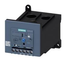
Overload relay 12.5...50 A Electronic For motor protection Size S3, Class 10E Stand-alone installation Main circuit: Straight-through transformer Auxiliary circuit: Screw Manual-Automatic-Reset
