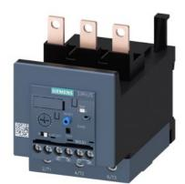
Overload relay 12.5...50 A Electronic For motor protection Size S3, Class 10E Contactor mounting Main circuit: Screw Auxiliary circuit: Screw Manual-Automatic-Reset
