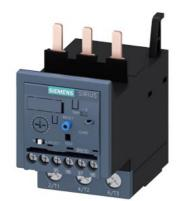
Overload relay 20...80 A Electronic For motor protection Size S2, Class 20E Contactor mounting Main circuit: Screw Auxiliary circuit: Screw Manual-Automatic-Reset
