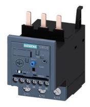
Overload relay 12.5...50 A Electronic For motor protection Size S2, Class 20E Contactor mounting Main circuit: Screw Auxiliary circuit: Screw Manual-Automatic-Reset
