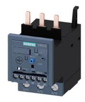
Overload relay 20...80 A Electronic For motor protection Size S2, Class 10E Contactor mounting Main circuit: Screw Auxiliary circuit: Screw Manual-Automatic-Reset
