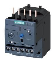
Overload relay 1...4 A Electronic For motor protection Size S00, Class 20E Contactor mounting Main circuit: Screw Auxiliary circuit: Screw Manual-Automatic-Reset
