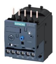
Overload relay 4...16 A Electronic For motor protection Size S00, Class 10E Contactor mounting Main circuit: Screw Auxiliary circuit: Screw Manual-Automatic-Reset
