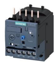
Overload relay 0.32...1.25 A Electronic For motor protection Size S00, Class 10E Contactor mounting Main circuit: Screw Auxiliary circuit: Screw Manual-Automatic-Reset
