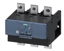
Overload relay 160...630 A for motor protection Size S10/S12, CLASS 5...30E Contactor mounting/stand-alone installation Main circuit: busbar connection Auxiliary circuit: Screw terminal Manual-Automatic-Reset Internal ground fault detection
