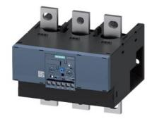
Overload relay 55...250 A for motor protection Size S10/S12, CLASS 5...30E Contactor mounting/stand-alone installation Main circuit: busbar connection Auxiliary circuit: Screw terminal Manual-Automatic-Reset Internal ground fault detection
