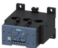
Overload relay 50...200 A for motor protection Size S6, CLASS 5...30E Contactor mounting/stand-alone installation Main circuit: straight-through transformer Auxiliary circuit: Screw terminal Manual-Automatic-Reset Internal ground fault detection
