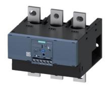
Overload relay 160...630 A for motor protection Size S10/S12, Class 20E Contactor mounting/stand-alone installation Main circuit: busbar connection Auxiliary circuit: Screw terminal Manual-Automatic-Reset
