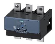
Overload relay 55...250 A for motor protection Size S10/S12, Class 10E Contactor mounting/stand-alone installation Main circuit: busbar connection Auxiliary circuit: Screw terminal Manual-Automatic-Reset
