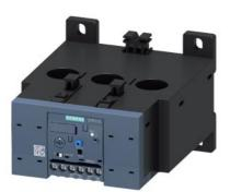
Overload relay 50...200 A for motor protection Size S6, Class 10E Contactor mounting/stand-alone installation Main circuit: straight-through transformer Auxiliary circuit: Screw terminal Manual-Automatic-Reset
