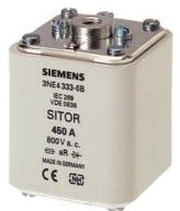
SITOR fuse link, with female thread on both sides, In: 500 A, aR, Un AC: 800 V, Un DC: 440 V, front indicator
