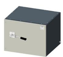
SINOVA, onload changeover switches 3KJ0, manually operated, size 5, 4-pole, in enclosed execution Iu: 2500 A, Ue AC: 415 V, Ie at AC-21 B at 415 V: 2300 A, screw mounting, front operating mechanism, at the left end, complete unit with door operating mechanism, Metallic handle, grey and black colour, flat terminal
