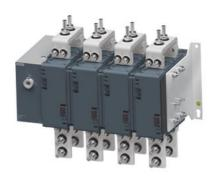
SINOVA, onload changeover switches 3KJ0, manually operated, size 4, 4-pole, in open execution, lu: 1250 A, Ue AC: 415 V, le at AC-22 A at 415 V: 1250 A, screw mounting, front operating mechanism, at the left end, complete unit with door operating mechanism, Metallic handle, grey and black colour, flat terminal
