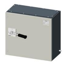
SINOVA, onload changeover switches 3KJ0, manually operated, size 4, 4-pole, in enclosed execution lu: 1000 A, Ue AC: 415 V, le at AC-22 A at 415 V: 1000 A, screw mounting, front operating mechanism, at the left end, complete unit with door operating mechanism, Metallic handle, grey and black colour, flat terminal
