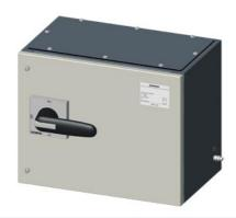
SINOVA, onload changeover switches 3KJ0, manually operated, size 2, 4-pole, in enclosed execution Iu: 200 A, Ue AC: 415 V, Ie at AC-23 A at 415 V: 200 A, screw mounting, front operating mechanism, at the left end, complete unit with door operating mechanism, Plastic handle, grey and black colour, flat terminal
