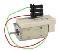
MN undervoltage release, Compact NS 630b to 3200, 200 VDC to 250 VDC, 200 VAC to 250 VAC 50/60 Hz
