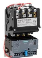
Non-reversing motor starter Size 0 Three phase full voltage Solid-state overload relay OLRelay amp range 5.5-22A 110-120/220-240VAC 60HZ coil Combination type No enclosure
