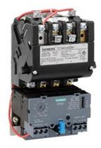
Non-reversing motor starter Size 0 Three phase full voltage Solid-state overload relay OLRelay amp range 3-12A 110-120/220-240VAC 60HZ coil Combination type No enclosure
